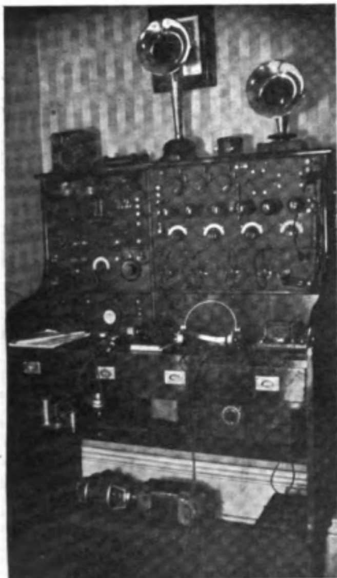
2 PV. Showing H.F. Intervalve Transformer in position.
